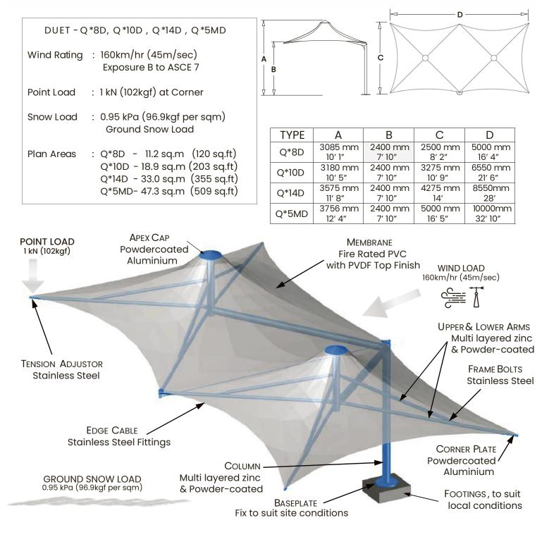
Flexshade® Quartet<sup>™</sup> can be designed to suit specific customer requirement for height and plan dimension.
